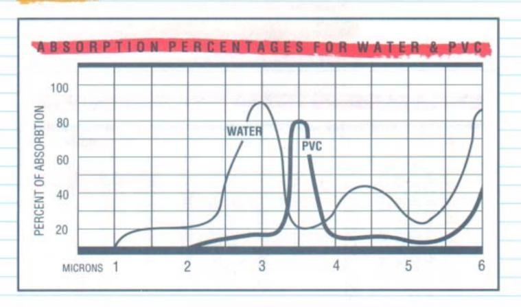
As an example, the above illustrates the difference in absorption curves for water and PVC. Find the peak absorption areas of the graph above. For most plastics, the CH (carbon/hydrogen) bond will peak in the 3.2 - 3.4 micron area. For water, the OH (oxygen/hydrogen) bond will peak at 2.9 - 3.0 micron area. Ideally, you would like your heater to output the majority of its energy in the area where it will be absorbed best.
