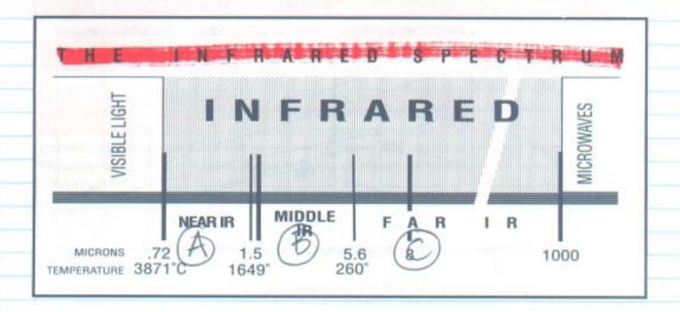
To determine whether a heater falls into the category of a short, medium or long infrared heater, 80% of your effective output should be within a defined range.
