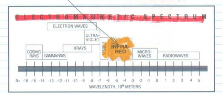
Find the infrared spectrum within the electromagnetic spectrum. Notice that it is bordered by the visible spectrum on one end and the microwave spectrum on the other. The infrared region ranges between .72 and 1,000 microns.
