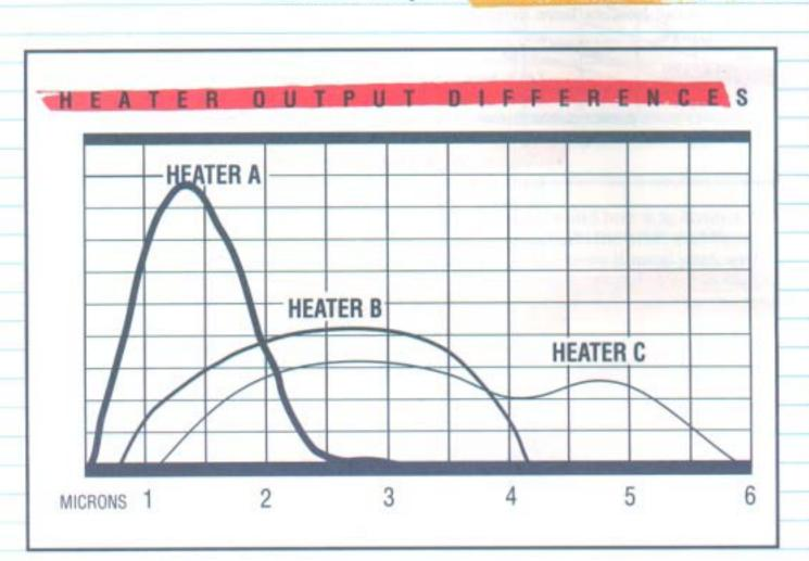
use a controller to regulate the temperature. From the above examples, we can conclude that same-watt heaters can deliver totally different outputs.
